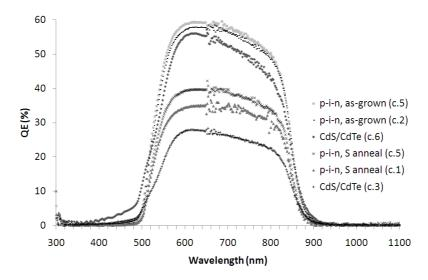
Fig. 3: QE characterisation of different contacts from devices incorporating  $FeS_x$  layers with and without S annealing, and for a p-n structure without the  $FeS_x$  layer.
