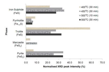
Fig. 1: Normalised XRD peak intensities to show proportional phases present in MOCVD FeS<sub>x</sub> layers on CdS after sulphurisation at temperatures  $400^{\circ}\text{C}$  -  $500^{\circ}\text{C}$ .
