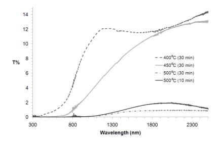
Fig. 2: Comparison of Transmittance spectra of FeS<sub>x</sub> deposited onto CdS at 300 °C by MOCVD with post-sulphurisation at temperatures 400 °C - 500 °C.
