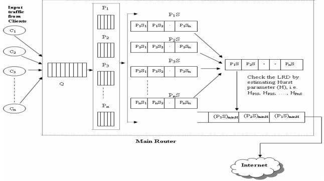
Fig. 1. Illustration of packets management for controlling LRD at router buffer
