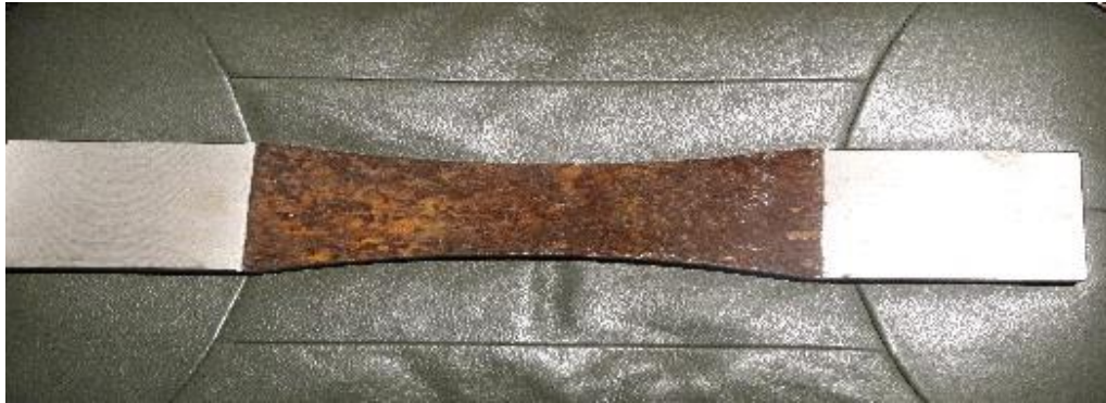
Figure 8 Corroded specimen prior to testing
