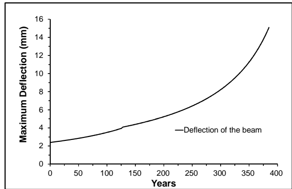
Figure 27 Bridge 44: a). Increase in maximum stress with time, b). Increase in maximum deflection with time
