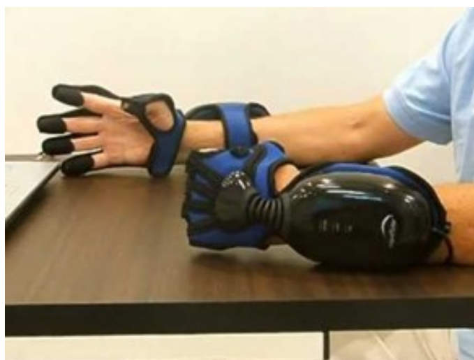
Fig. 2. HandTutor fingers rehabilitation glove.
