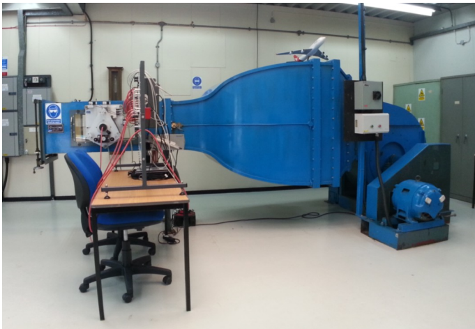
Fig. 4. Subsonic wind tunnel for the experimental research.
