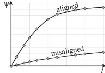
Fig. 3. Magnetisation curves for aligned and misaligned positions.
