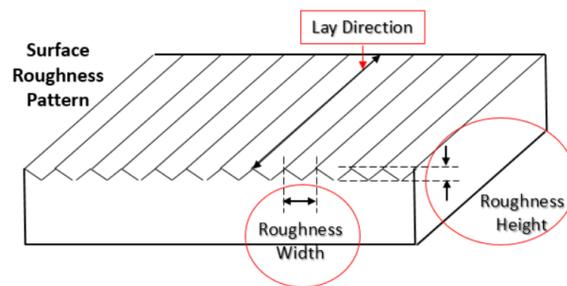
Figure 1: surface characteristics
