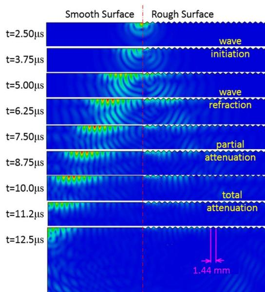
Figure 7: surface wave attenuation where  $\lambda_{\text{surface}} / \lambda_{\text{wave}} = 0.5$
