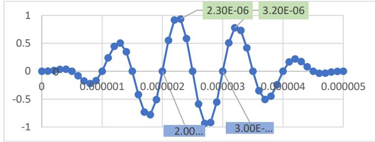
Figure 3: Hanning windowed incident wave signal at  $T = 1 \mu\text{s} \rightarrow f = 1 \text{ MHz}$ .
