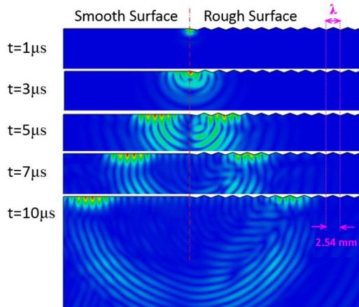
Figure 6: surface wave propagation where  $\lambda_{\text{surface}} / \lambda_{\text{wave}} = 1$
