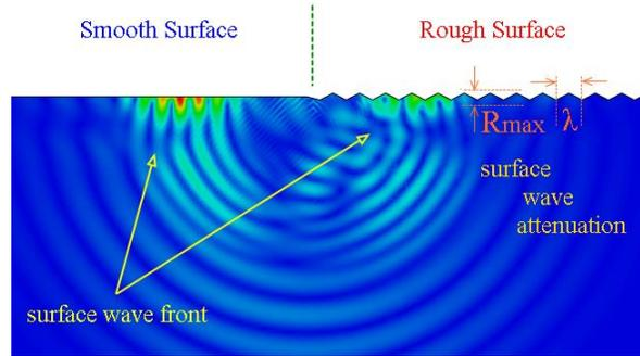
Figure 5: Rayleigh wave propagation on smooth surface vs. rough surface
