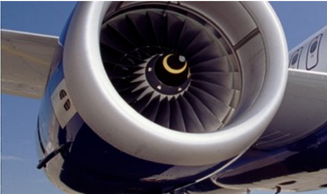
Fig. 3. IAE V2500-A5 aircraft engine fan [4].
