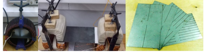
Fig. 7. Experimental setups and the steel rectangular lamination samples.
