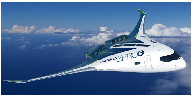
Fig. 9. Airbus ZEROe BWB, distributed thrust concept aircraft [18].
