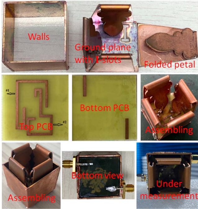
Fig. 5. Fabricated prototype of the proposed dual-polarized bowtie antenna.
