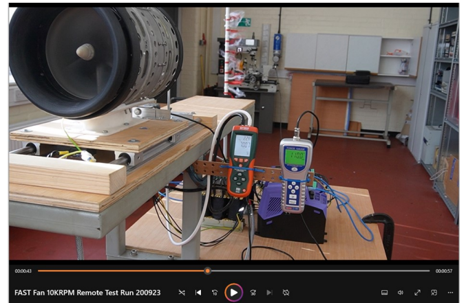
Fig. 6. Still image taken from the test video of the Fast-fan operating at the maximum test speed of 10,000 rpm.
