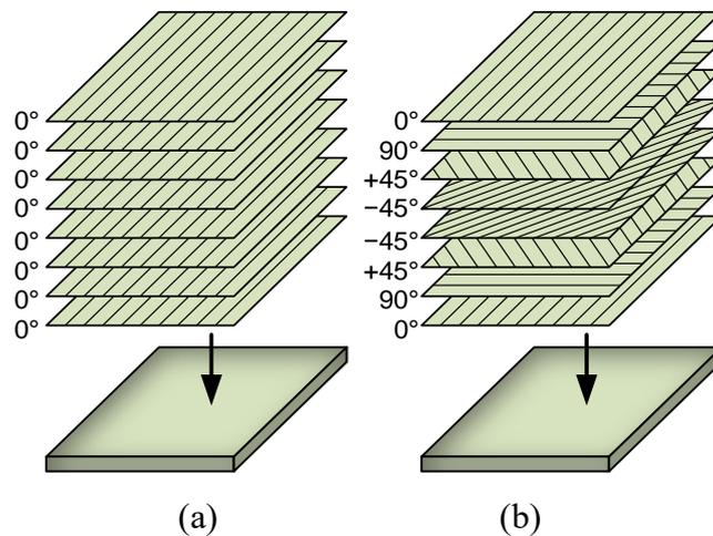
**Figure 2. Ply stacking sequence of a fibre-reinforced composite: (a) unidirectional, (b) cross-plyed quasi-isotropic.**
