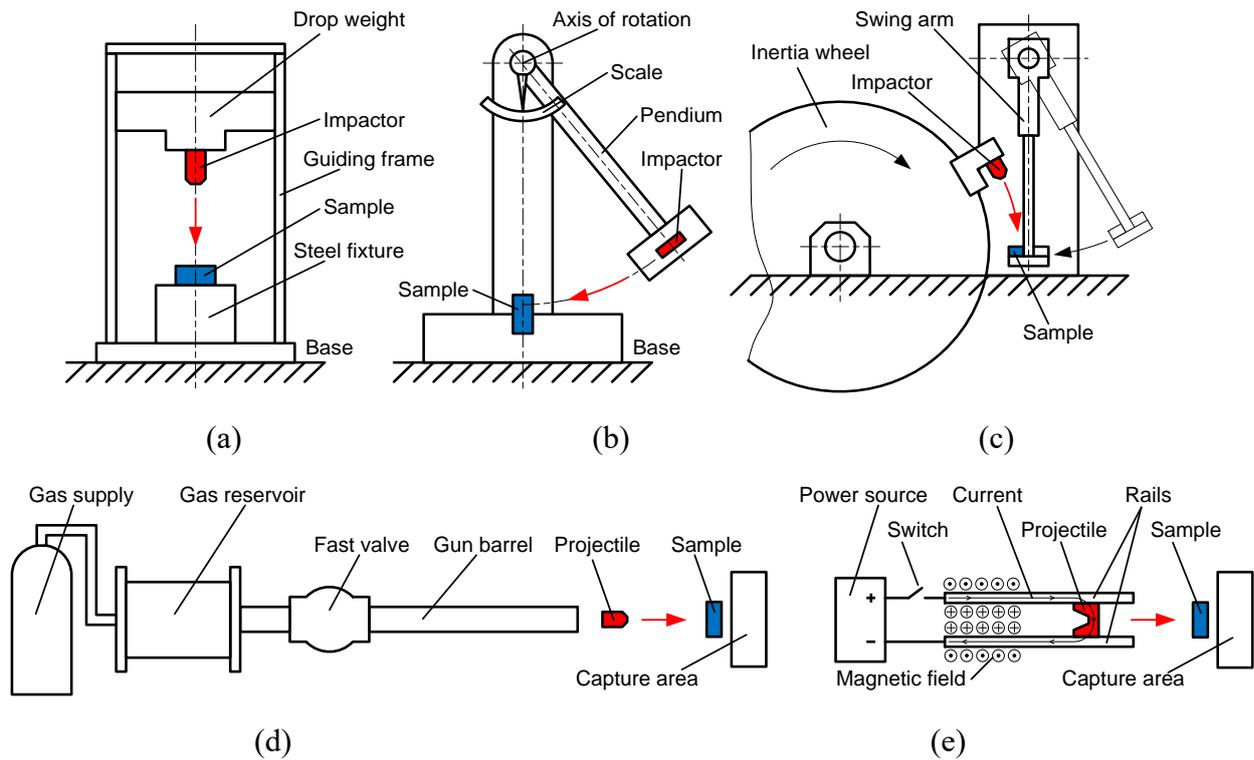
**Figure 4. Schematic of impact testing methods; (a) drop weight impact testing, (b) pendulum impact testing, (c) inertia wheel impact testing, (d) gas gun impact testing, (e) electromagnetic launcher impact testing.**
