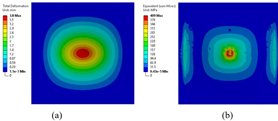
Figure 7. Total deformation and von Mises stress contours during impact on unidirectional composite laminate: (a) front side total deformation; (b) rear side von Mises stress.
