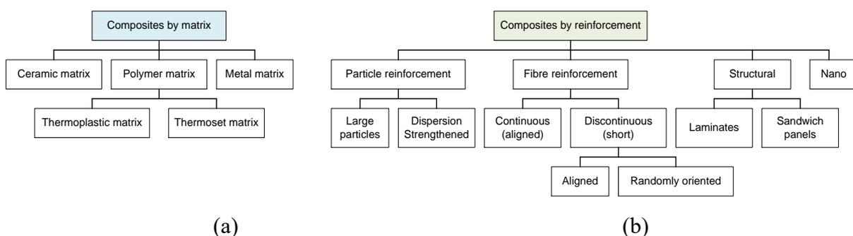
**Figure 1. Classification of composites by (a) matrix and (b) reinforcement.**
