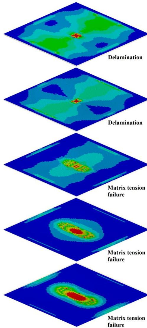
Figure 6. Composite laminate failure of different unidirectional plies after spherical impact from above.
