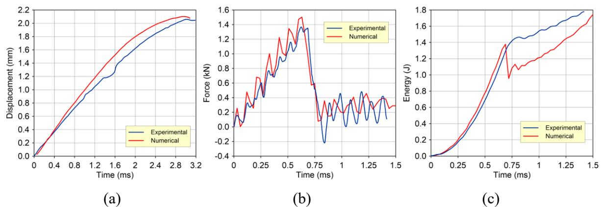
**Figure 5. Experimental and numerical comparisons of displacement, force, and energy versus time; (a) spherical impact on curved GFRP composite plate, data from (Seifoori et al. 2021), (b) cylindrical impact on [0/90]<sub>3s</sub> GFRP laminate plate, data from (Boukar et al. 2022), (c) cylindrical impact on [0/90]<sub>3s</sub> GFRP laminate plate, data from (Boukar et al. 2022).**
