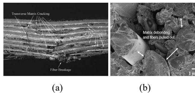
**Figure 3. Damage and failure modes of composite materials; (a) delamination, matrix cracking, and fibre breakage (Saeedifar et al. 2018), (b) matrix debonding and fibre pull-out (Hernandez et al. 2017).**
