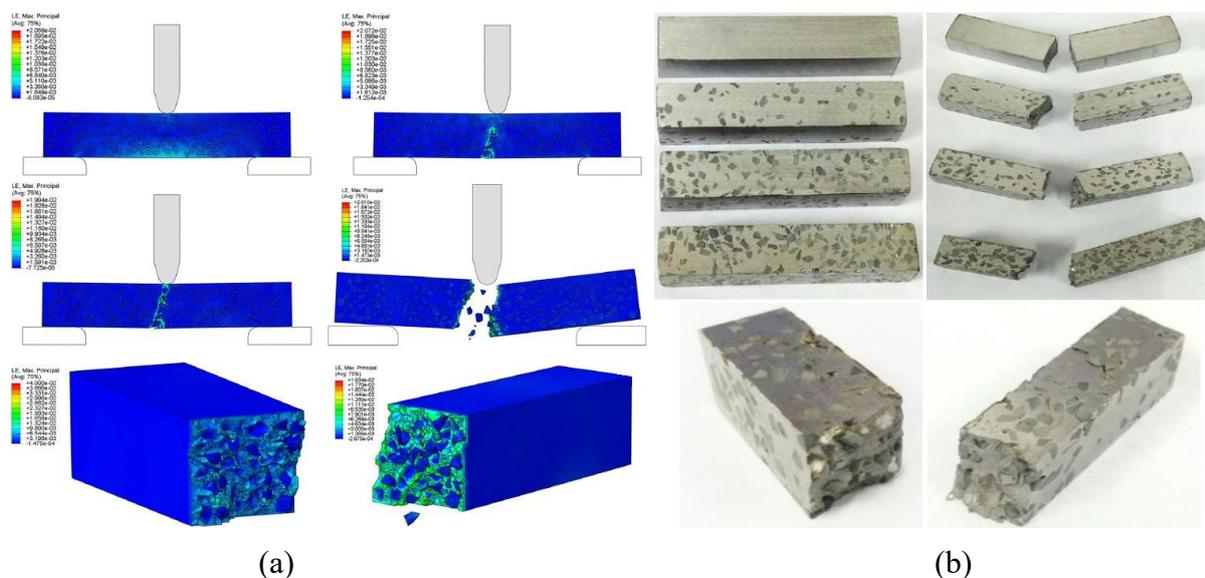
Figure 8. Charpy impact test on particle reinforced MMC test specimen (Miao et al. 2022): (a) simulated fracture progress; (b) experimental specimen and fracture.
