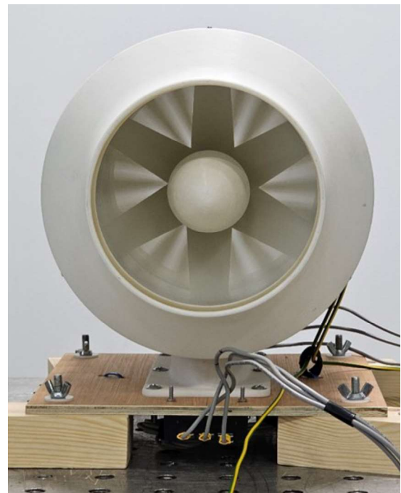
Fig. 1. Prototype Fast-Fan device, viewed on the exhaust nozzle, whilst undergoing laboratory testing.
