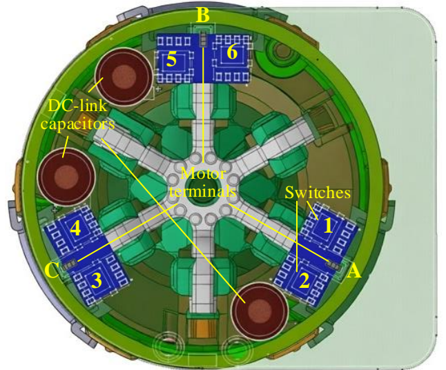
Fig. 7. Design of inverter PCB.
