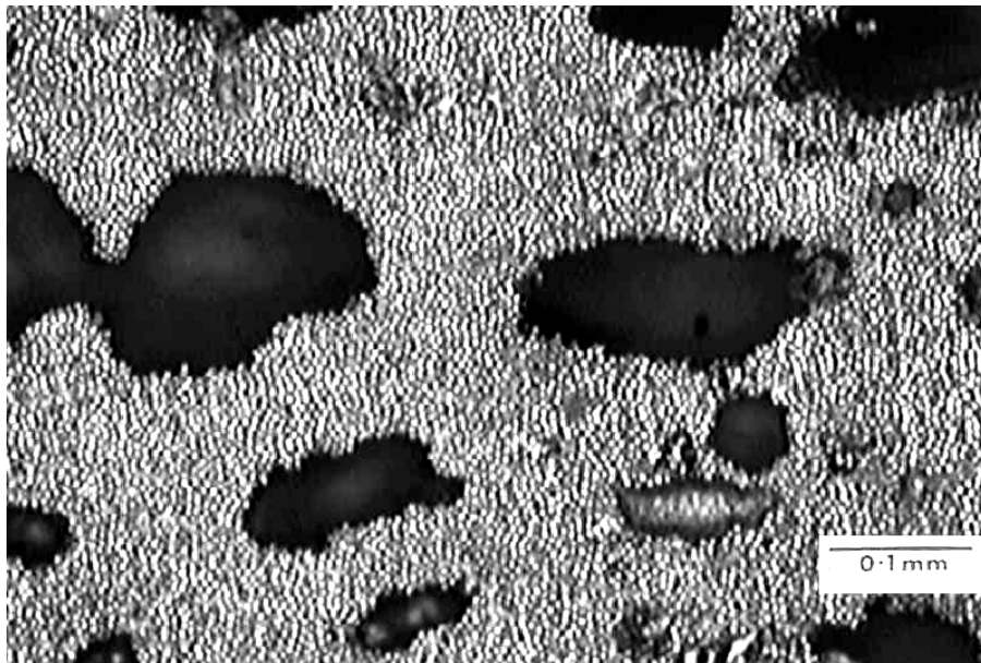
Figure 13. Microwave cured System 1 composite, fibres perpendicular to radius of turntable
