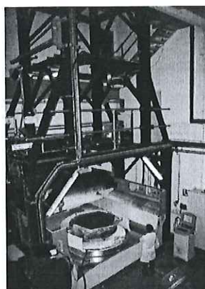
Fig. 2 Zeeko machine under OTT for in-situ full-aperture interferometry
