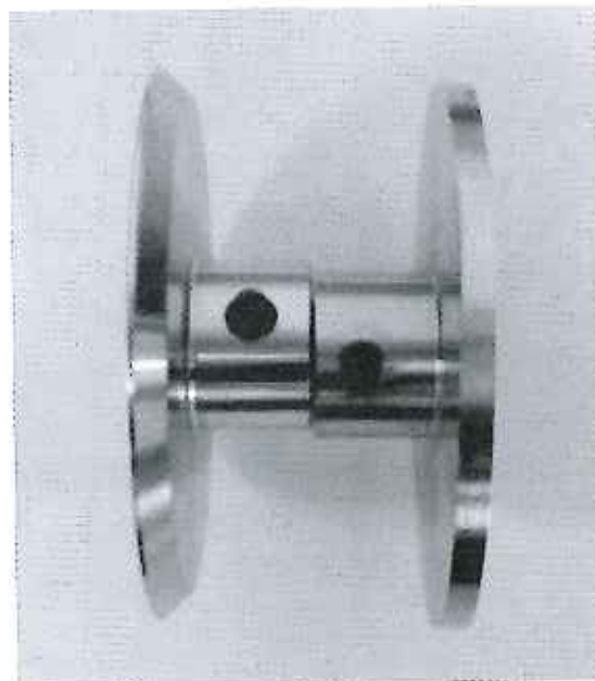
Figure 15. Two rotating discs of thickness t' = 0.5\text{ mm} and 3\text{ mm} (left and right respectively)
