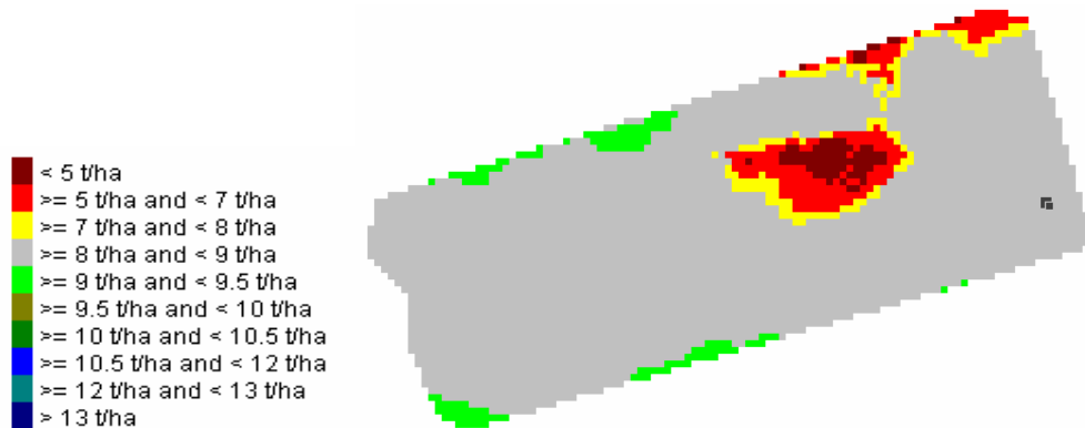
Fig. 8. Actual wheat yield map obtained from a GPS-enabled combine harvester in the August 2003 harvest for “ Ben’s Field ” at the Riseholme Park Farm. (Wheat variety: “ Tanker ”).
